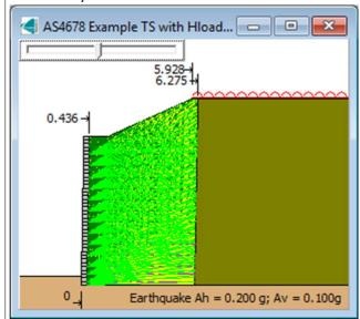
An H load of 30 kN/m is added to the section above, using the parameters in the first image. Partial load factors of relevance in AS4678 are as follows:
